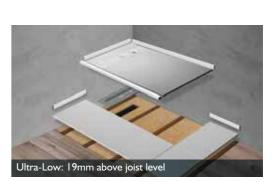
(Additional waterproof floor area at same level) Flooring removed to desired area and false floor created at joist level.
