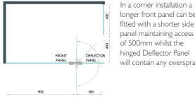
longer front panel can be fitted with a shorter side panel maintaining access of 500mm whilst the hinged Deflector Panel will contain any overspray.
